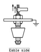
No traction exerted on the wires
