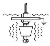
Make sure ther are no vibrations in the installation area A specific request is otherwise necessary
