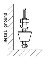
Do not install in the vicinity of a magnetic metal ground Risk of modification or disturbance in the detection
