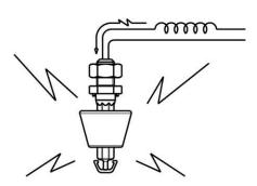
Check the kind of electric load on the contacts The value indicated on the drawing is for a resistive load only!
