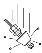
Avoid any shock to the level sensor when stored or when fitted as it may otherwise modify its characteristics
