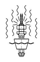
Check the water tightness between the float assembly and the cable assembly
