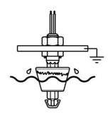
Make sure the chemical character of the liquid used is compatible with the components of the sensor that are immersed, in combination with the operating or peak temperature and the required lifetime
