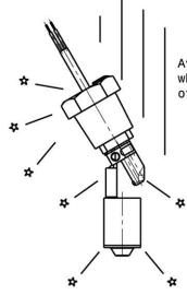
Avoid any shock to the level sensor when stored or when fitted as it may otherwise modify its characteristics
