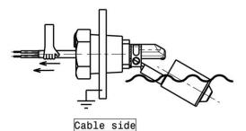
No traction exerted on the wires
