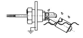
Make sure the chemical character of the liquid used is compatible with the components of the sensor that are immersed, in combination with the operating or peak temperature and the required lifetime
