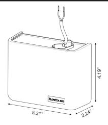
Hose diameter (internal) Discharge: 0.23" - not supplied
