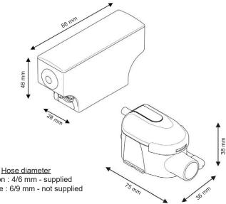
Hose diameter Suction : 4/6 mm - supplied Discharge : 6/9 mm - not supplied
