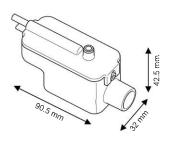
Hose diameter Suction: 6/9 mm - not supplied Discharge: 6/9 mm - not supplied
